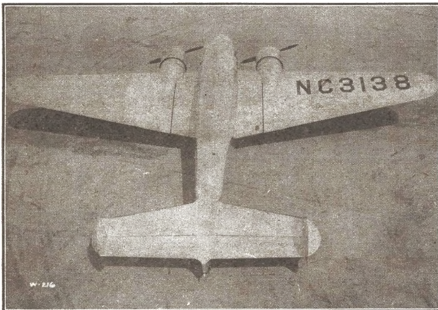
Here's the real Lockheed Electra poised on the runway ready for a scheduled hop. The Electra, which is built principally of Alclad 24st., a high-strength duralumin, is a ten-passenger job capable of better than 200 m.p.h. As you construct your model, check it with this photo and you won't go wrong.
